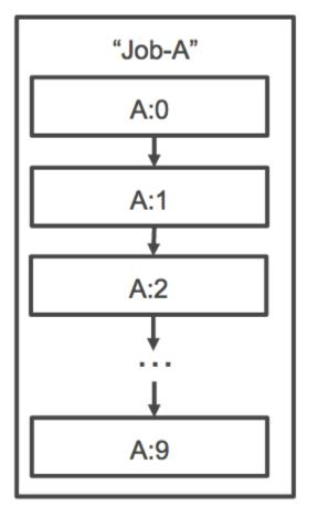
You can also specify an N\_TO\_N type dependency with a job ID for array jobs. That way, each index child of this job must wait for the corresponding index child of each dependency to complete before it can begin. The following figure shows Job A and Job B, two array jobs with an array size
