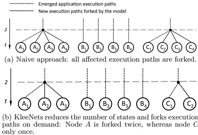
**Figure 4:** Comparison of the naive approach and optimizations provided by KleeNet.
