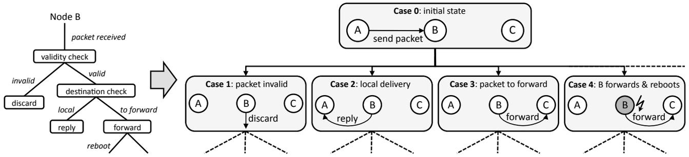
**Figure 1: KleeNet’s debugging approach.** The initial execution path (*A* broadcasts a packet to *B*) splits after packet reception at node *B* into four execution paths: packet invalid, local delivery, packet to forward, and packet to forward followed by a reboot of node *B*. Following these execution paths, KleeNet provides a high program coverage including non-deterministic failures such as reboots and packet losses.
