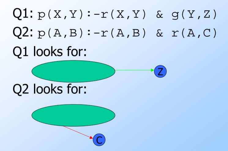
**Example --- Continued** And not every subgoal Q1: p(X,Y):-r(X,Y) & q(Y,Z)need be a target. Q2: p(A,B):-r(A,B) & r(A,C)Notice two subgoals can Containment mapping: m(A)=X; map to one. m(B)=m(C)=Y.
