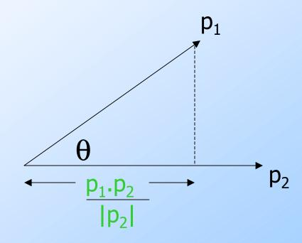
d (p<sub>1</sub>, p<sub>2</sub>) =  $\theta$  = arccos(p<sub>1</sub>.p<sub>2</sub>/|p<sub>2</sub>||p<sub>1</sub>|)
