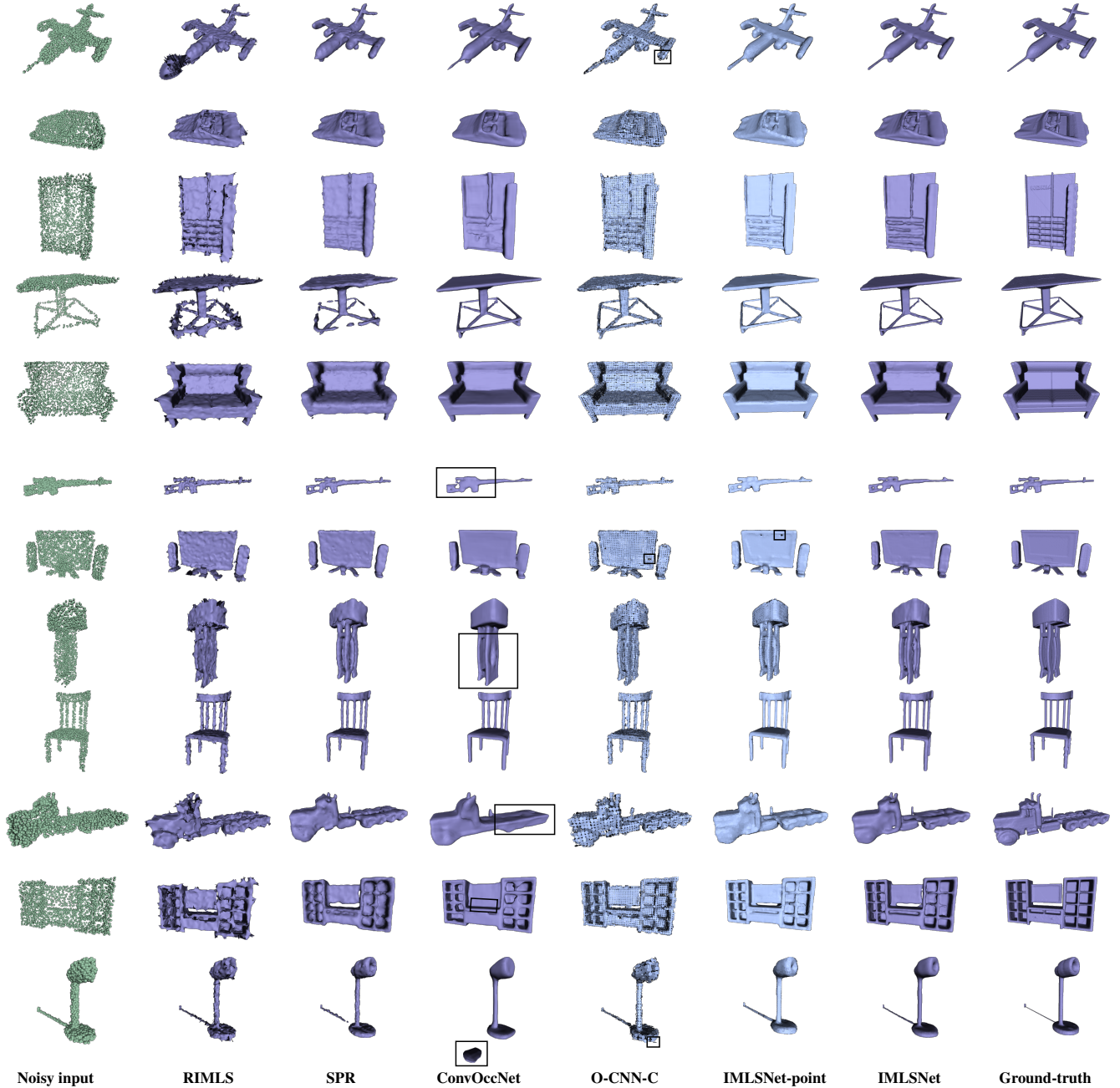
Figure 3: Visual results of 3D object reconstruction from point clouds by different methods. For point outputs of O-CNN-C and IMLSNet-point, we render points as oriented disks. Some artifacts in the results are labeled by black boxes.
