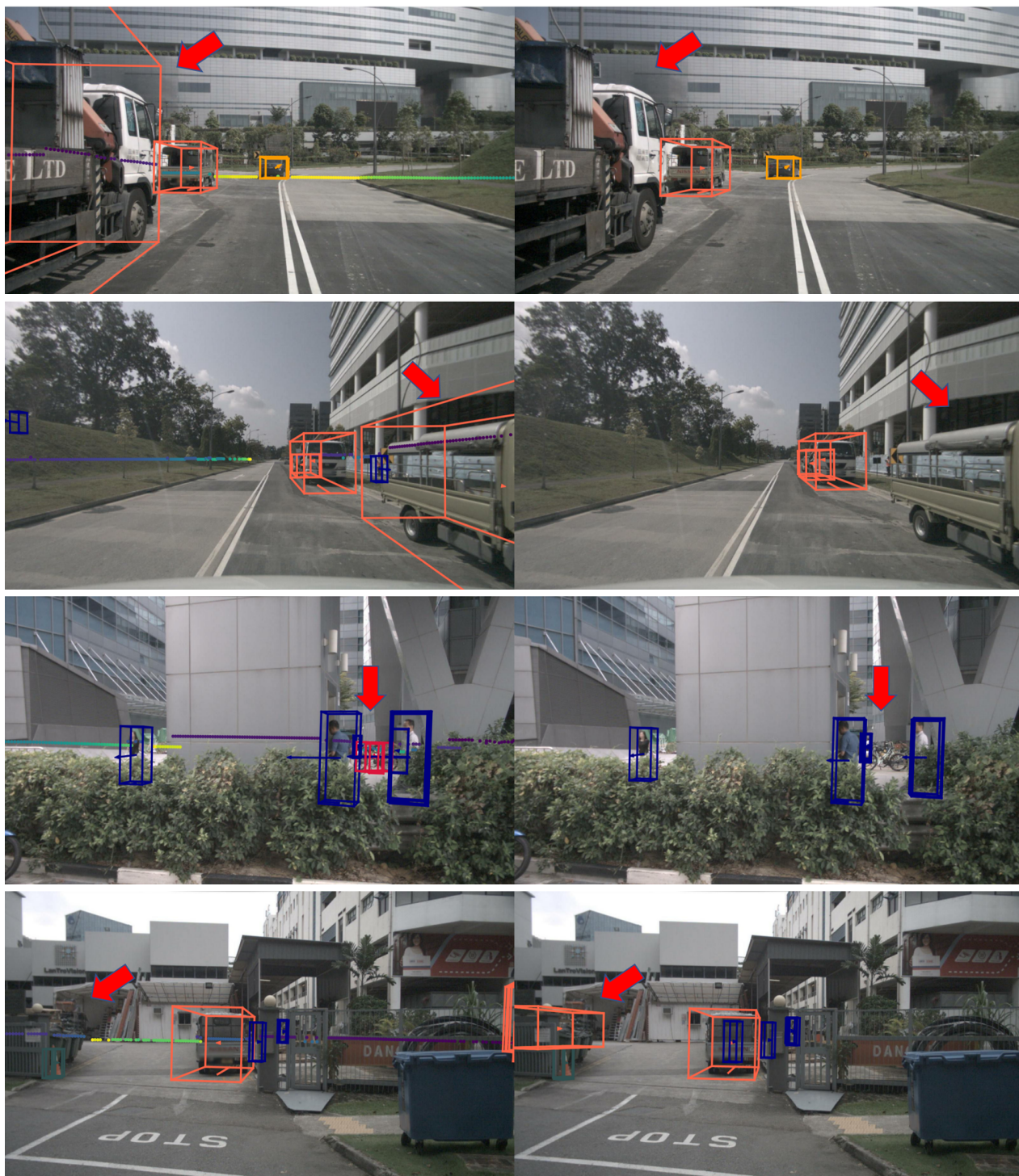
Figure B. Results visualization in perspective images. On the left is 1-beam LiDAR with cameras, on the right is cameras. Even sparse points like 1-beam LiDAR can help FUTR3D to detect and correct the false positive.
