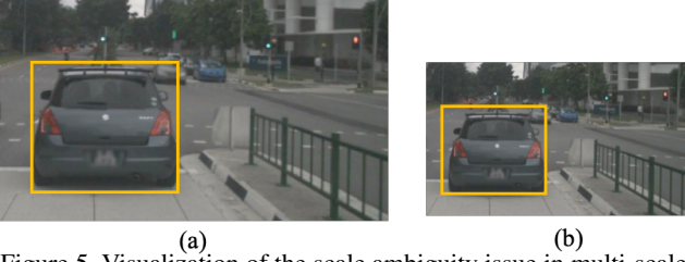
Figure 5. Visualization of the scale ambiguity issue in multi-scale training. Though the number of image pixels inside the yellow box in (a) and (b) varies, the supervision remains the same.
