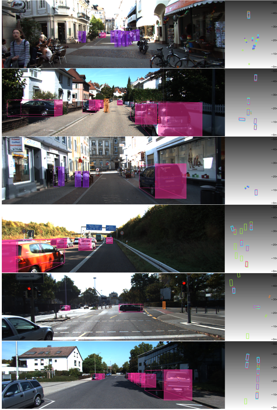
Fig. 13: KITTI Qualitative Results. DEVIANT predictions in general are more accurate than GUP Net [49]. [Key: Cars, Cyclists and Pedestrians of DEVIANT; all classes of GUP Net, and Ground Truth in BEV].
