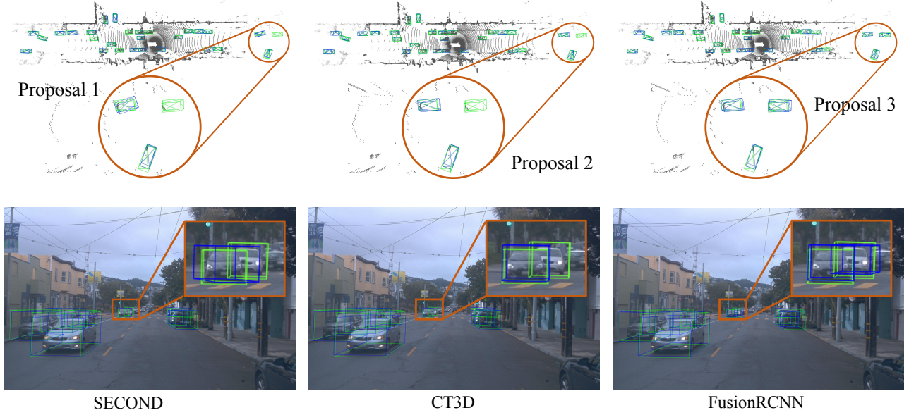
Fig. 3. Qualitative comparison between LiDAR-based two-stage detector (CT3D) and our FusionRCNN on the Waymo Open Dataset. Green boxes and Blue boxes are ground-truth and prediction, respectively. Three proposal vehicles in red circle are zoom-in and visualize on 2D images and 3D point clouds. Our FusionRCNN works better than CT3D with only LiDAR input in long range detection.
