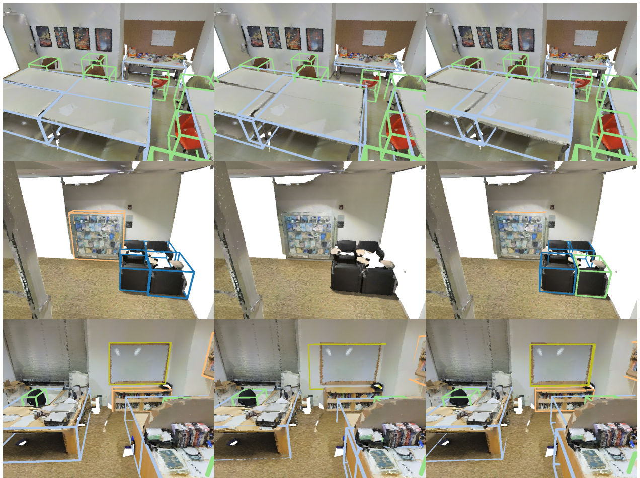
Figure 7. Visual Comparison on S3DIS 3D detection. Left: Ground-truth. Middle: FCAF3D's result. Right: SWIN3D-L+FCAF3D's results.
