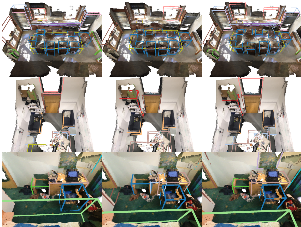
Figure 6. Visual comparison of ScanNet 3D detection. Left: Ground truth. Middle: FCAF3D’s result. Right: SWIN3D-L+CAGroup3D’s results. Note that the original CAGroup3D paper does not release its checkpoint, so no visual results provided in this figure.
