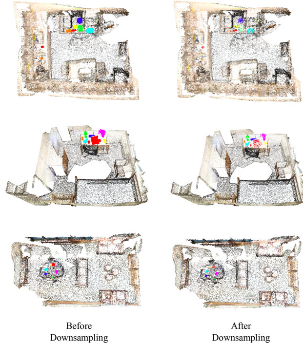
Fig. 11: Visualization of scenes in TO-SCENE before (originally provided in [50]) and after (our TO-SCENE-down benchmark) downsampling. After downsampling, the density of points on small objects is closer to others, which is more realistic.
