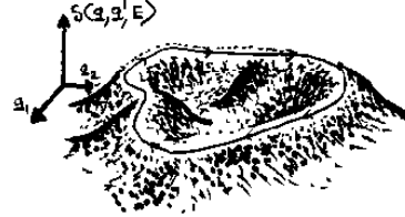
Figure 39.2: A romanticized sketch of S_p(E) = S(q, q, E) = \oint p(q, E) dq landscape orbit. Unstable periodic orbits traverse isolated ridges and saddles of the mountainous landscape of the action S(q_{||}, q_{\perp}, E) . Along a periodic orbit S_p(E) is constant; in the transverse directions it generically changes quadratically.
