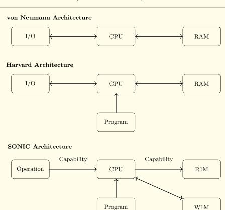
The architecture uses zk-AluVM virtual machine, immutable memory cells of two types (read-once memory, R1M; and write-once memory, W1M), and capability-based R1M access.
