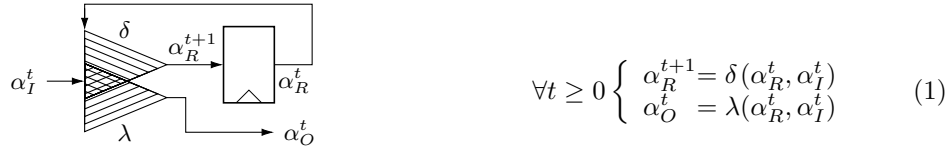
Figure 2: Functional Mealy machine.
